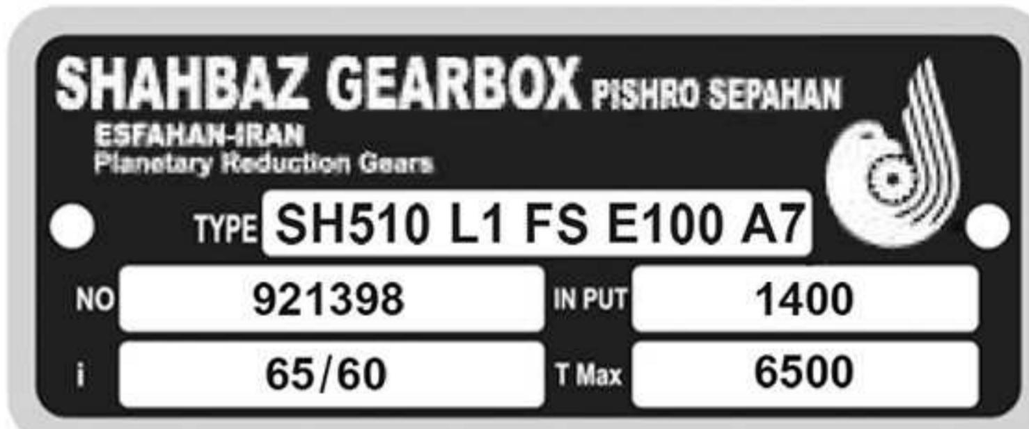
Solar gearboxes are identified by following properties and signs.
